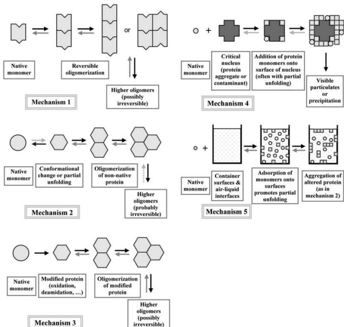
Figure 3: Schematic illustration of five common aggregation mechanisms. Taken from Philo et al. 2009<sup>20</sup>
