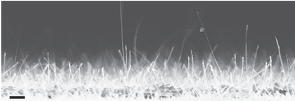
Figure 1. SEM micrograph of a Si NW support where the presence of NWs with different lengths can be observed. Stage tilting 54°. Scale bar 1 \mu\text{m} .
