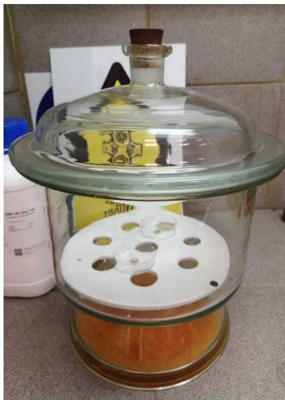
Figure 10. Functionalised mica stored in a desiccator.
