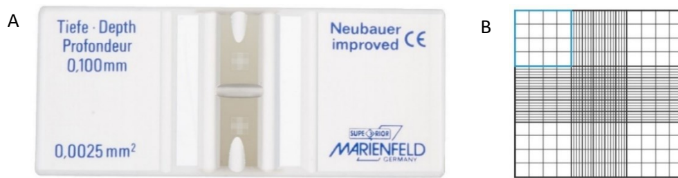
Figure 7. A) Neubauer chamber used for cell viability assessment; B) gridline indicating one of the sets of 16 squares used for counting cells 42
