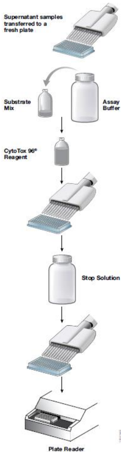
Figure 9. The Cytotox 96 ® Non- Radioactive Cytotoxicity Assay protocol. Supernatant samples were transferred to a 96 well plate and an equal volume of Cytotox 96 ® Reagent was added to each well and incubated for 30 minutes. Stop Solution was added, and absorbance signal was measured at 490 nm in a plate reader. "Retrieved from: Promega Corporation, "CytoTox 96 Non-Radioactive Cytotoxicity Assay," Promega Tech. Bull. 163, pp. 1-14, 1999."
