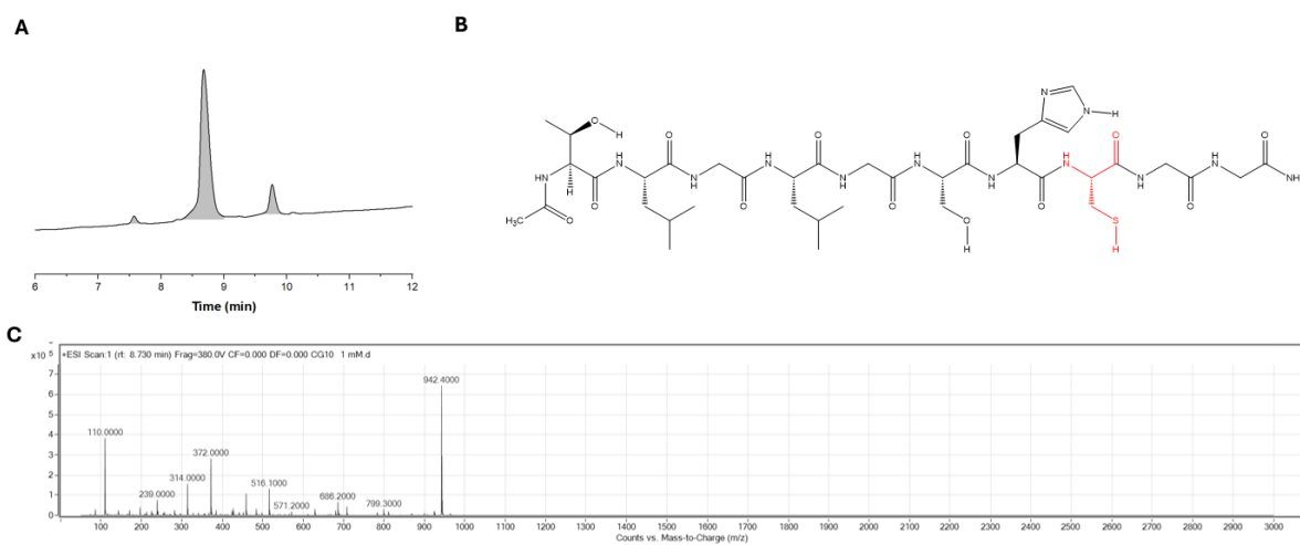
Supplementary Figure S4: a) LC chromatogram at 220 nm (purity of 89%), b) chemical structure and (c) the MS trace for Ac-TLGLGSHCGG-Am (CG10) ( m/z 941.4)
